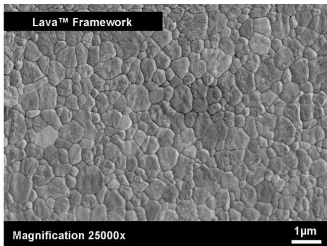
SEM of polycrystalline structure of Lava<sup>™</sup> Framework  $ZrO_2$  (mean particle size about 0.6  $\mu m$ ).
