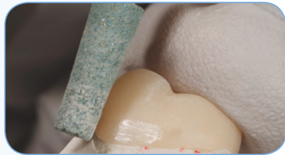
Gross contouring of full ZrO 2 crown with green coarse LD Grinder LD13C.
