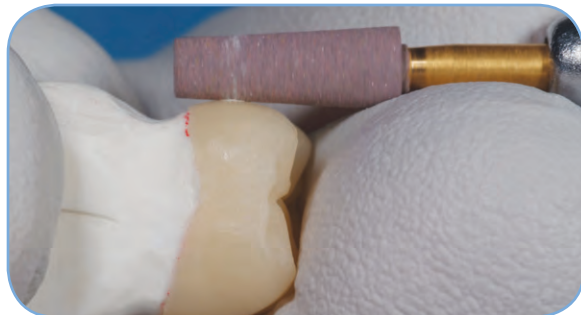
Grinding off positioning sprue with LD Grinder LD13M, which minimizes heat generation.
