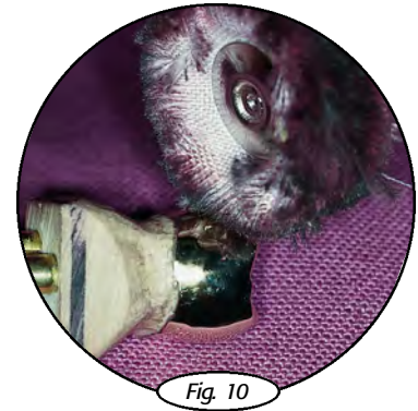
A 16422HP muslin high-shine rag wheel with rouge is used to put the final high-shine on the gold crown.
