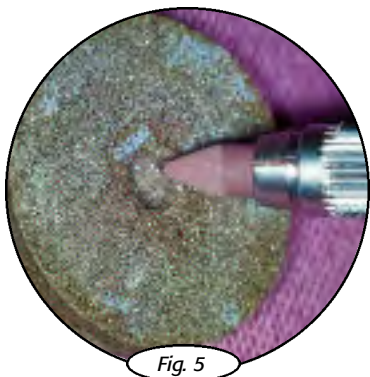
Fig. 5 Using an 1108 dressing stone (not included in kit) shape the 1102-030 red cylinder into a small point and smooth the central pit and deep fossa.
